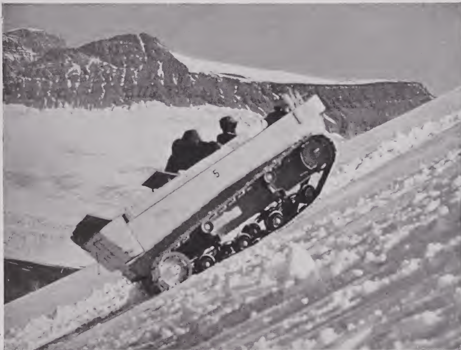
FIGURE 27. Pilot model of T-15 Weasel climbing 20-degree slope on Mount Castleguard. Columbia Ice Fields.
